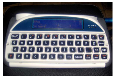
Figure 50: Lightwriter text-based AAC device
