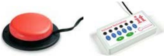
Figure 46: A switch and USB switch interface to connect it to a computer
