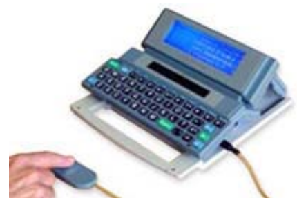
Figure 51: Lightwriter with switch access
