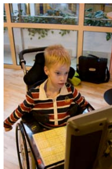
Figure 26: A learner using an eye-gaze voice output communication aid
